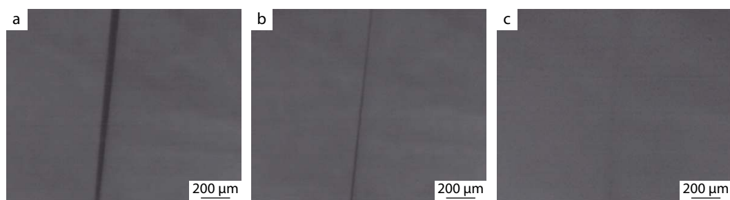
Fig. 10 Optical microscopic images of cracked EDBS-2 sample healing for various time: (a) 0 h, (b) 1.5 h, and (c) 3 h.
